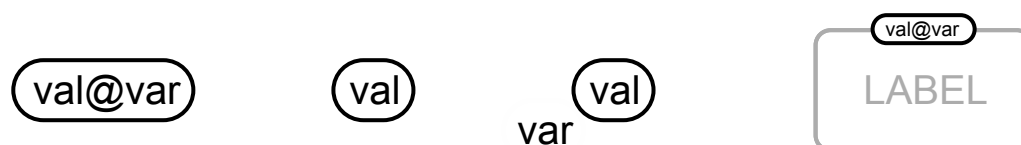
Figure 2.3: The Process Description glyph for state variable, shown with a value and a variable on the far left, with only a value on the middle-left, with an additional label for the variable on the middle-right (discouraged), and decorating a macromolecule (Section 2.4.3) on the far right.
